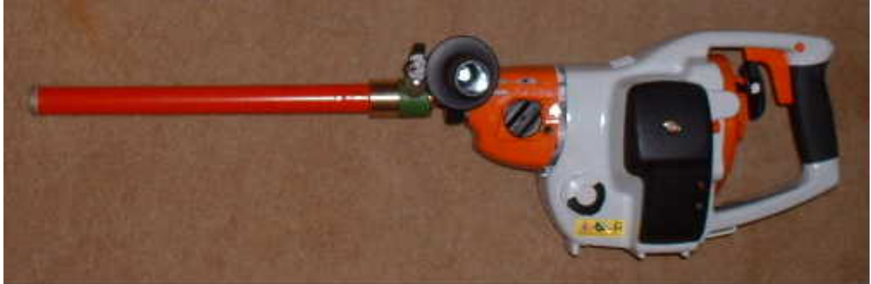
MMPRD Portable Rock Drill and 1" diamond corer.
