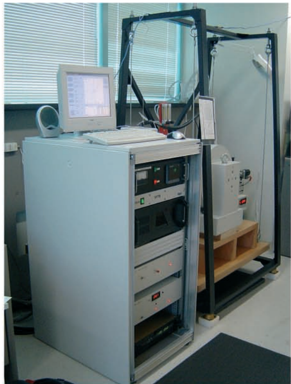
MM VFTB ELECTROMAGNET at Dr. Emilio Herrero-Bervera's laboratory, Institute of Geophysics and Planetology, University Of Honolulu, Hawaii, USA
