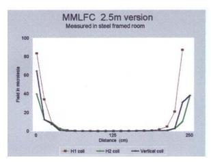
Adjustable. When magnetic materials (computers, magnetometers etc.) are placed inside a shielded room they generate magnetic fields. With solid steel shielded rooms these 'internal' magnetic fields are trapped INSIDE the room. The MMLFC with its electronic control system can be adjusted to compensate for internal fields and ensure the lowest field conditions for your samples. Ideal for eliminating viscous magnetisation (VRM) acquisition during experiments.
