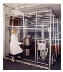
**Power and size.** The MMLFC can be supplied in any size up to 2.5 m x 2.5 m x 2.5 m. Power consumption is <0.75KVA and 110 or 240V versions are available. The 3 axis fluxgate has a noise level of 3nT and alignment of better than  $0.1^{\circ}$ .
